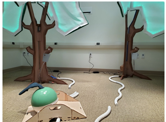
Fig. 1. MAPLE, showing two trees, the bridge, pipeline connectors, and our robot, “Maple” featuring a “floppy-ear” that conveys emotions. Not shown are a third tree and the “syrup bucket.” (See Fig. 3 for the complete MAPLE).
